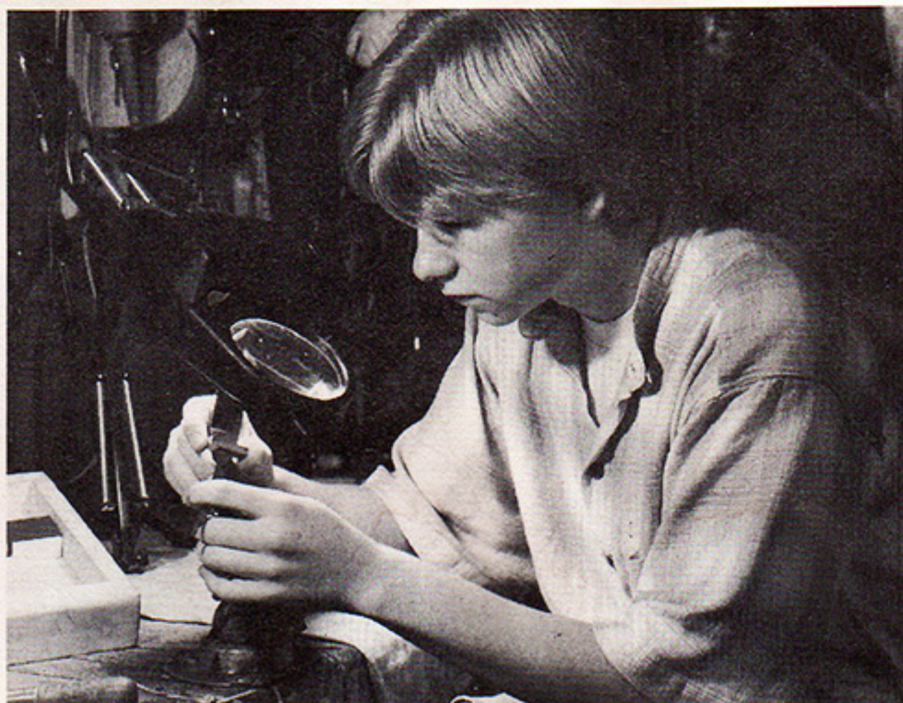
Gavin Hawk pays special attention to hand fitting a guard on one of his knives, through use of a microscope.
