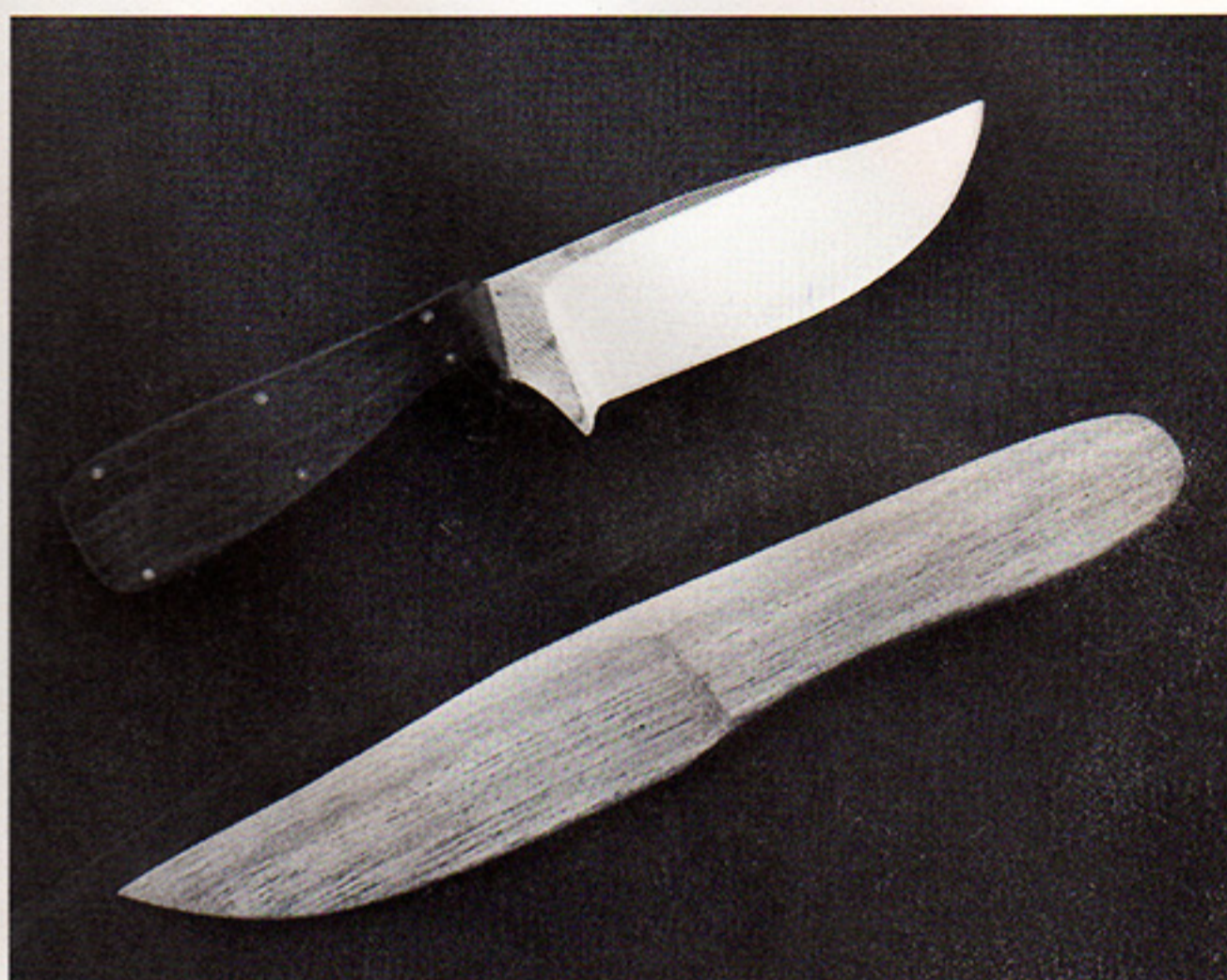
Hours of making wooden knives taught Gavin how to achieve an acceptable grind line on his first knife made from a file.
